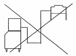
When installing condenser below the ice machine
